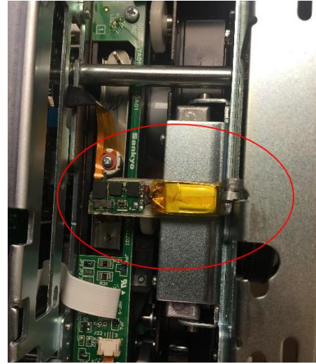
Skimmer attached below card reader - viewed from below
